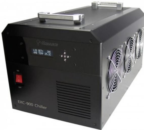
Koolance's EXC-900 is a portable recirculating liquid chiller rated at 900W, or 3071 BTU/hr (@25°C liquid & ambient). Chiller control is based on one of four configurable temperature set-points, including the option to lock liquid to ambient for avoiding condensation or to an external K-type thermocouple sensor (not included).
